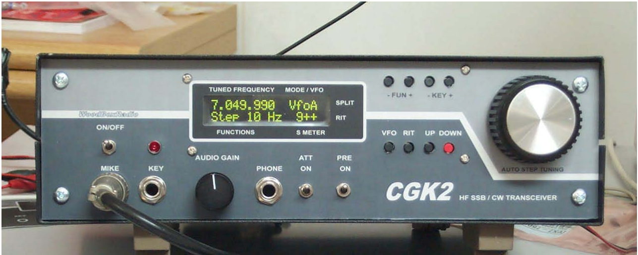
My all bands transceiver 1.8 -30 MHz (traditional one conversion using DDS instead of PLL )
