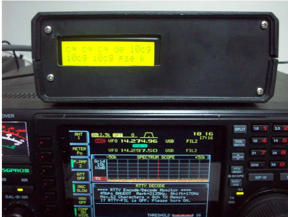
RTTY interface inside a prototype box in use with I0CG IC-756proIII
