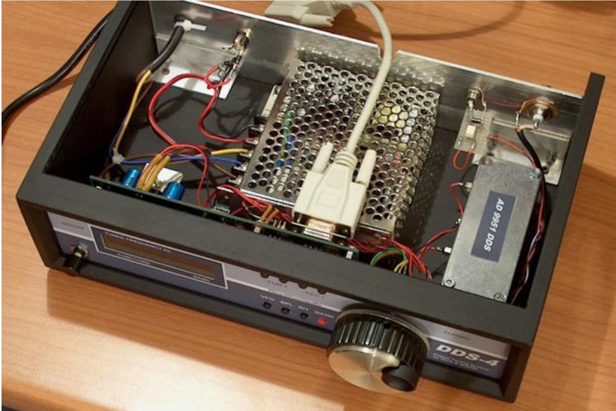
Close the top cover and connect the serial cable to one free COM PORT of your PC. Now your DDS-4 is ready for PC remote control
