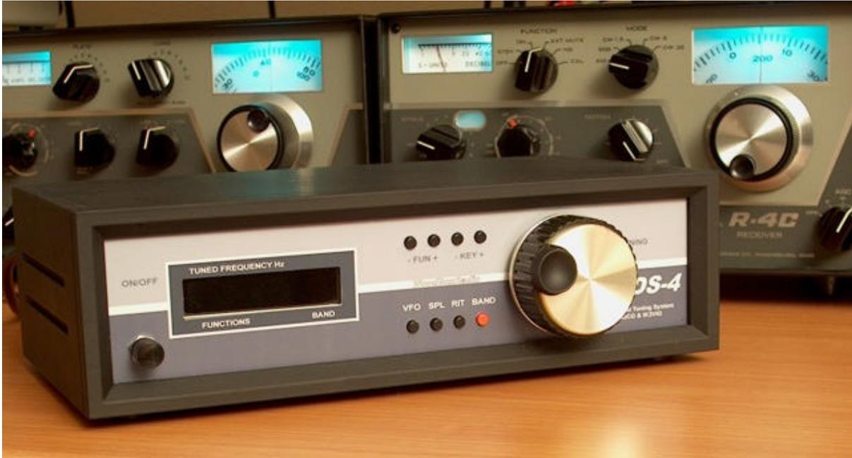
The DDS-4 is a complete Digital Tuning System, a VFO, with full control of DRAKE R4 receivers and T4 transmitter. It use a modern DDS AD9951 frequency generator and a PIC microcontroller.
